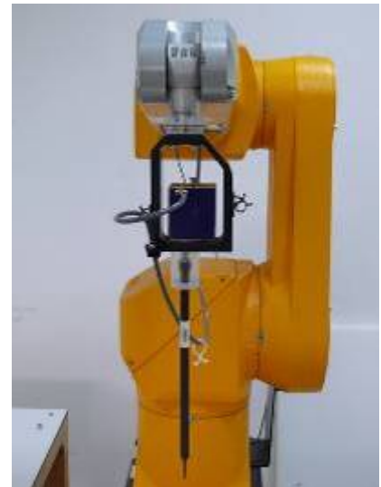
Figure 3. EX3DV4 E-field probe
