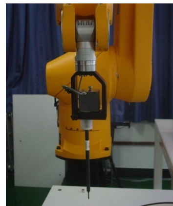
Picture 7.3 E-field Probe
