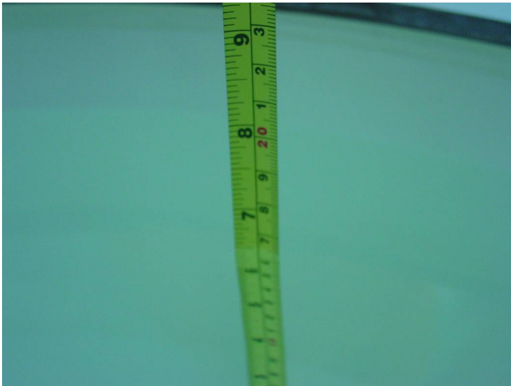
Picture 9.3 Liquid depth in the Flat Phantom (2450MHz)
