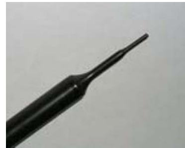
Picture 7.2 Near-field Probe
