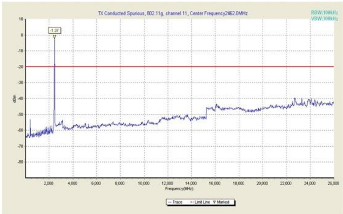
Fig. 28 Conducted Spurious Emission (802.11g, Ch11, 30 MHz-26 GHz)
