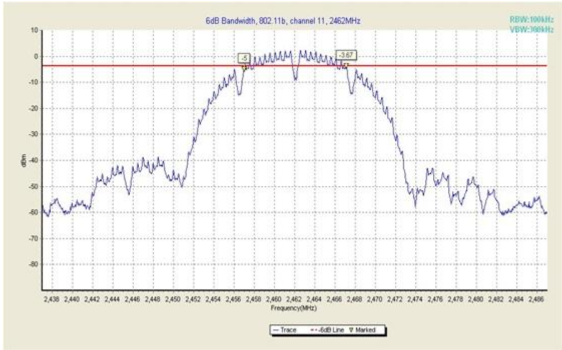
Fig. 9 Occupied 6dB Bandwidth (802.11b, Ch 11)
