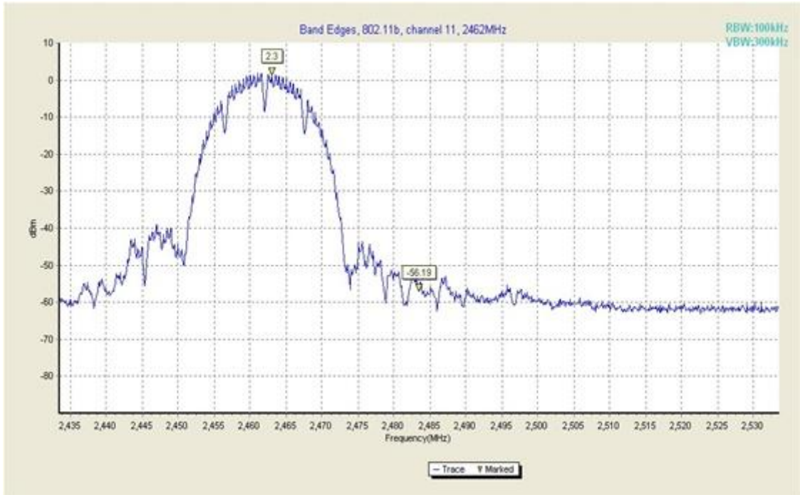
Fig. 14 Band Edges (802.11b, Ch 11)
