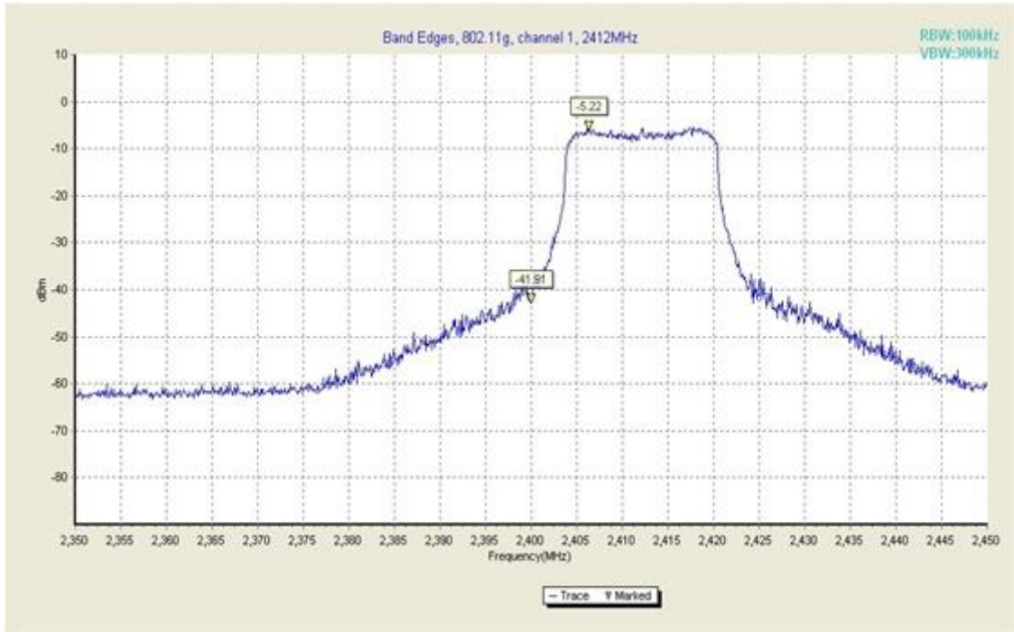
Fig. 15 Band Edges (802.11g, Ch 1)
