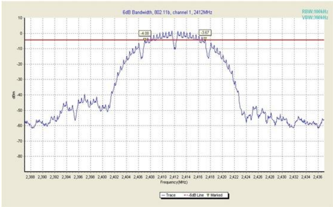
Fig. 7 Occupied 6dB Bandwidth (802.11b, Ch 1)
