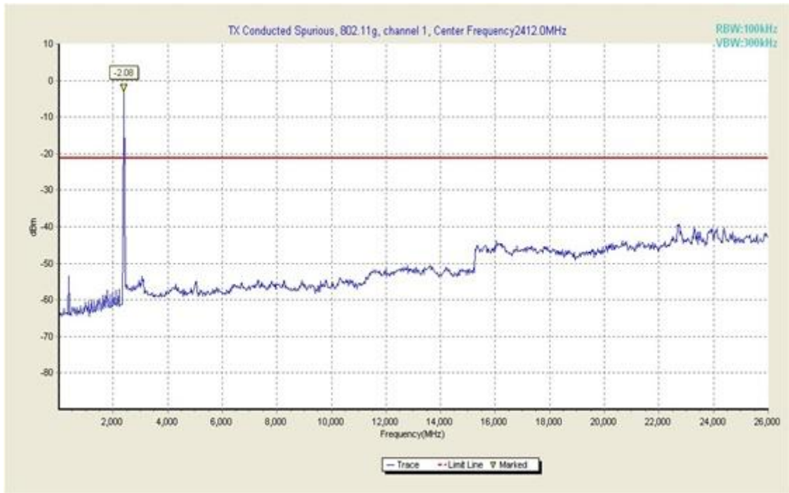
Fig. 24 Conducted Spurious Emission (802.11g, Ch1, 30 MHz-26 GHz)
