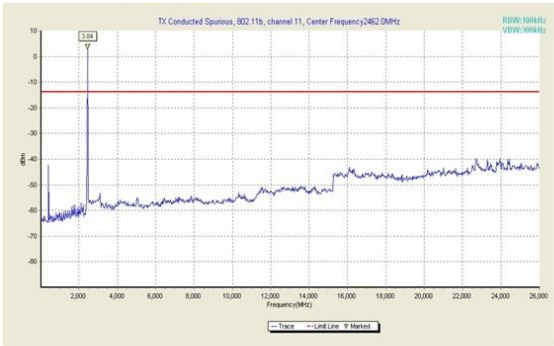
Fig. 22 Conducted Spurious Emission (802.11b, Ch11, 30 MHz-26 GHz)
