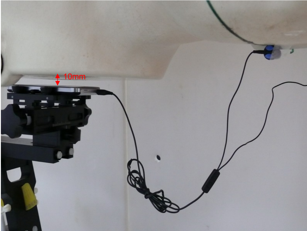
Picture 23: Front Side with Stereo Headset 3, the distance from handset to the bottom of the Phantom is 10mm
