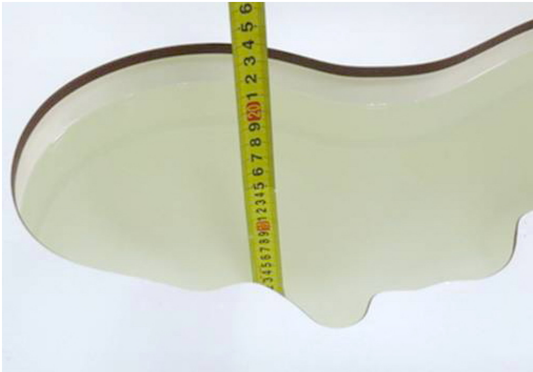
Picture 4: Liquid depth in the head Phantom (1750 MHz, 15.2cm depth)
