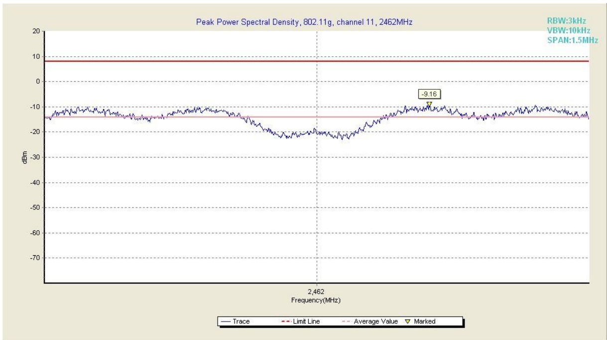
Fig. 6 Power Spectral Density (802.11g, Ch 11)
