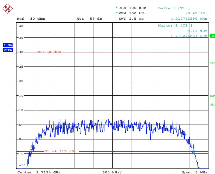
**Channel 1450-Occupied Bandwidth Reference Level**
