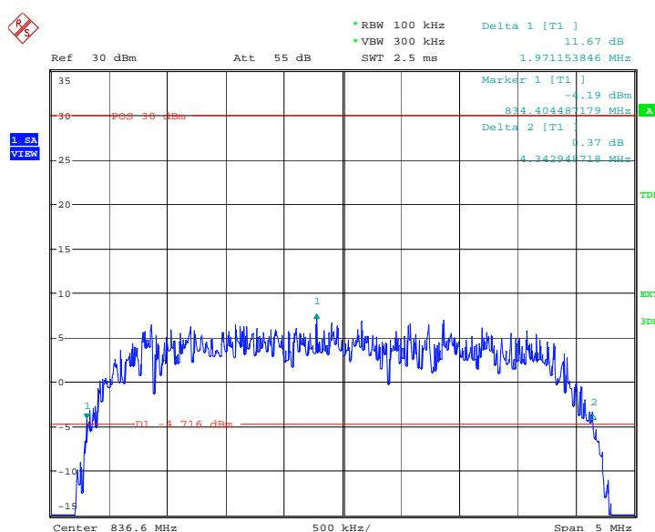
**Channel 4233-OccUPIed Bandwidth Reference Level**
