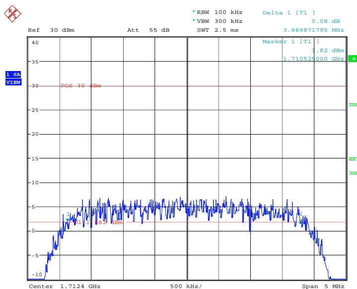
**Channel 1450-Occupied Bandwidth Reference Level**
