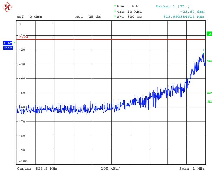
**HIGH BAND EDGE BLOCK-C (GSM850) –Channel 251**
