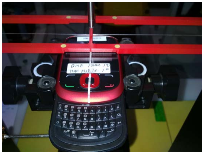
Picture 3: EUT Positioning for T-coil
