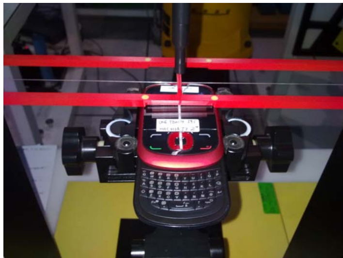
Picture 2: EUT Positioning for RF
