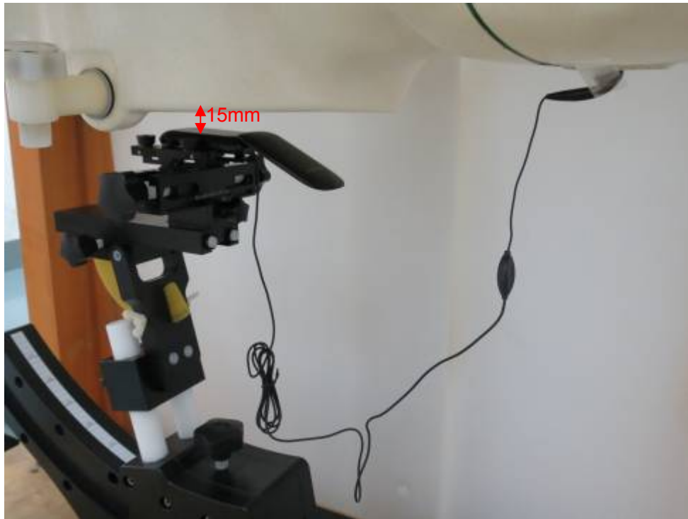
Picture 15: Body with Stereo Headset 2, The EUT towards ground, the distance from EUT to the bottom of the Phantom is 15mm (Cover Open)
