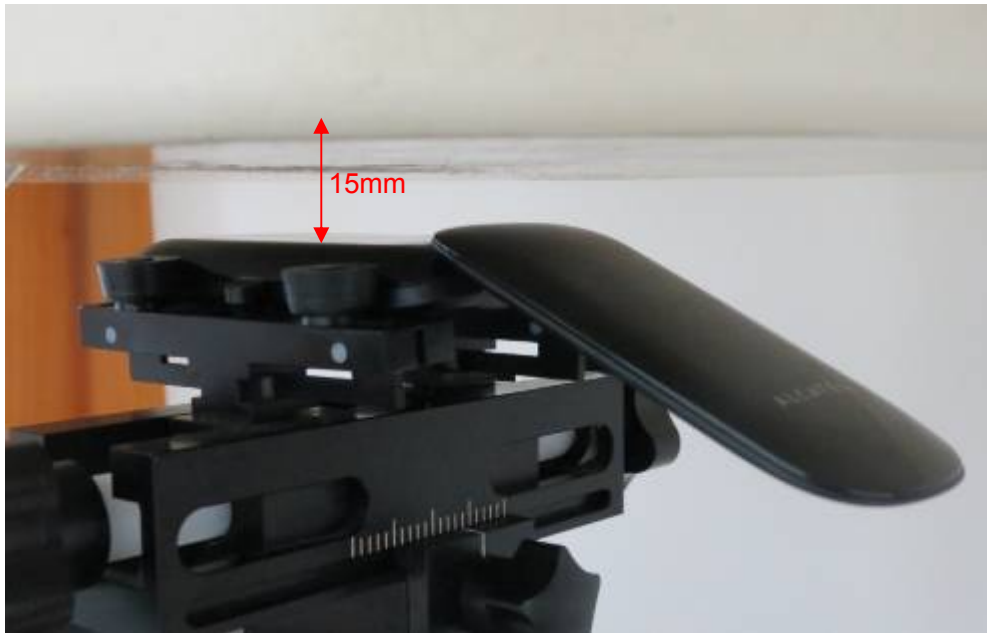
Picture 13: Body, The EUT towards ground, the distance from EUT to the bottom of the Phantom is 15mm (Cover Open)
