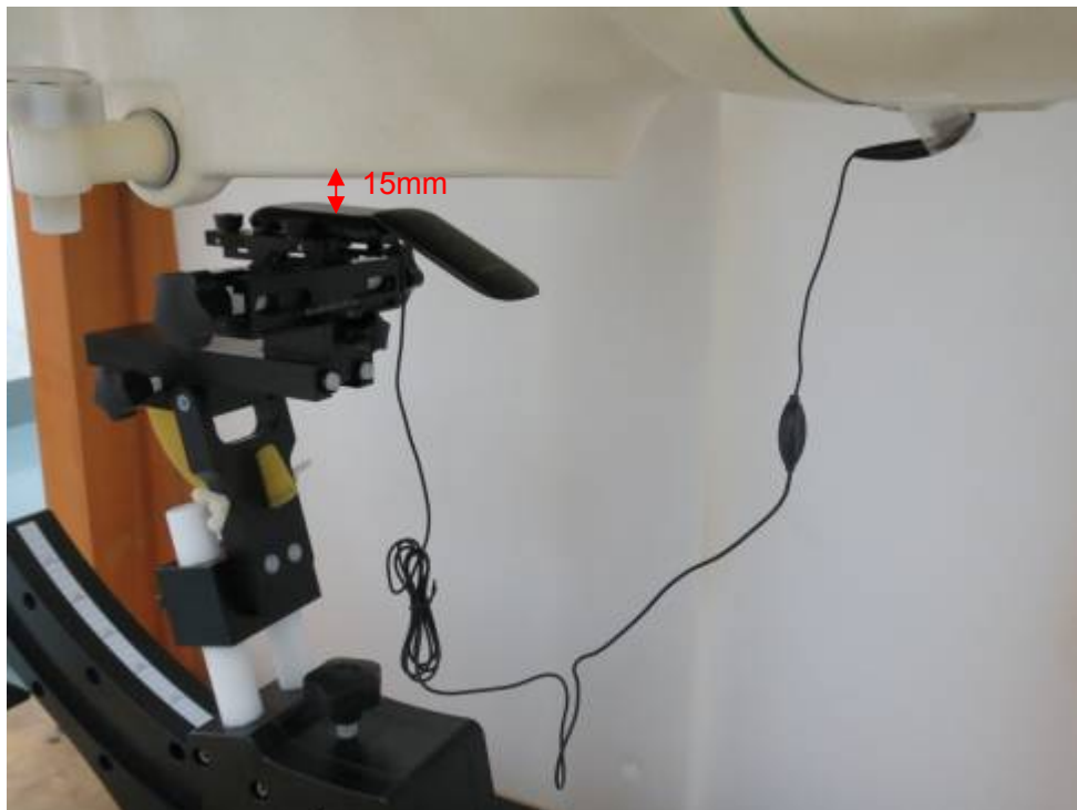
Picture 14: Body with Stereo Headset 1, The EUT towards ground, the distance from EUT to the bottom of the Phantom is 15mm (Cover Open)
