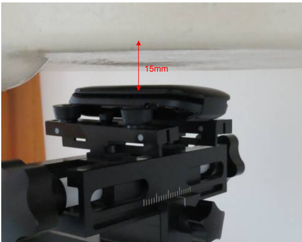
Picture 12: Body, The EUT towards phantom, the distance from EUT to the bottom of the Phantom is 15mm (Cover Close)
