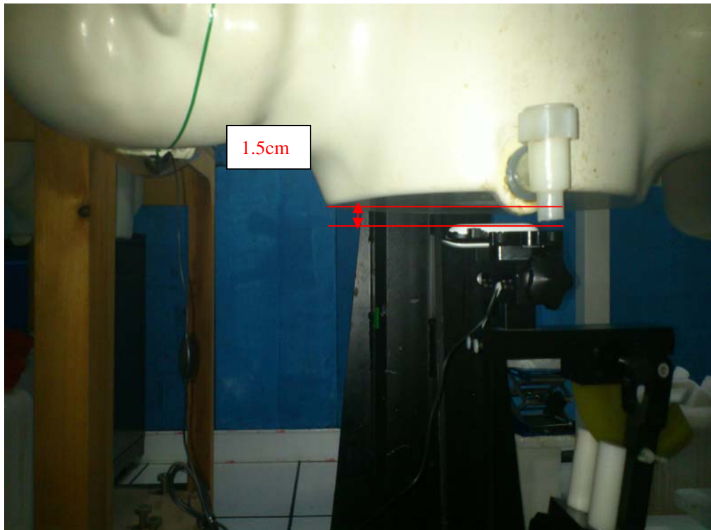
Picture B10: Body-worn Position with Headset (towards ground, the distance from handset to the bottom of the Phantom is 1.5cm) - folded
