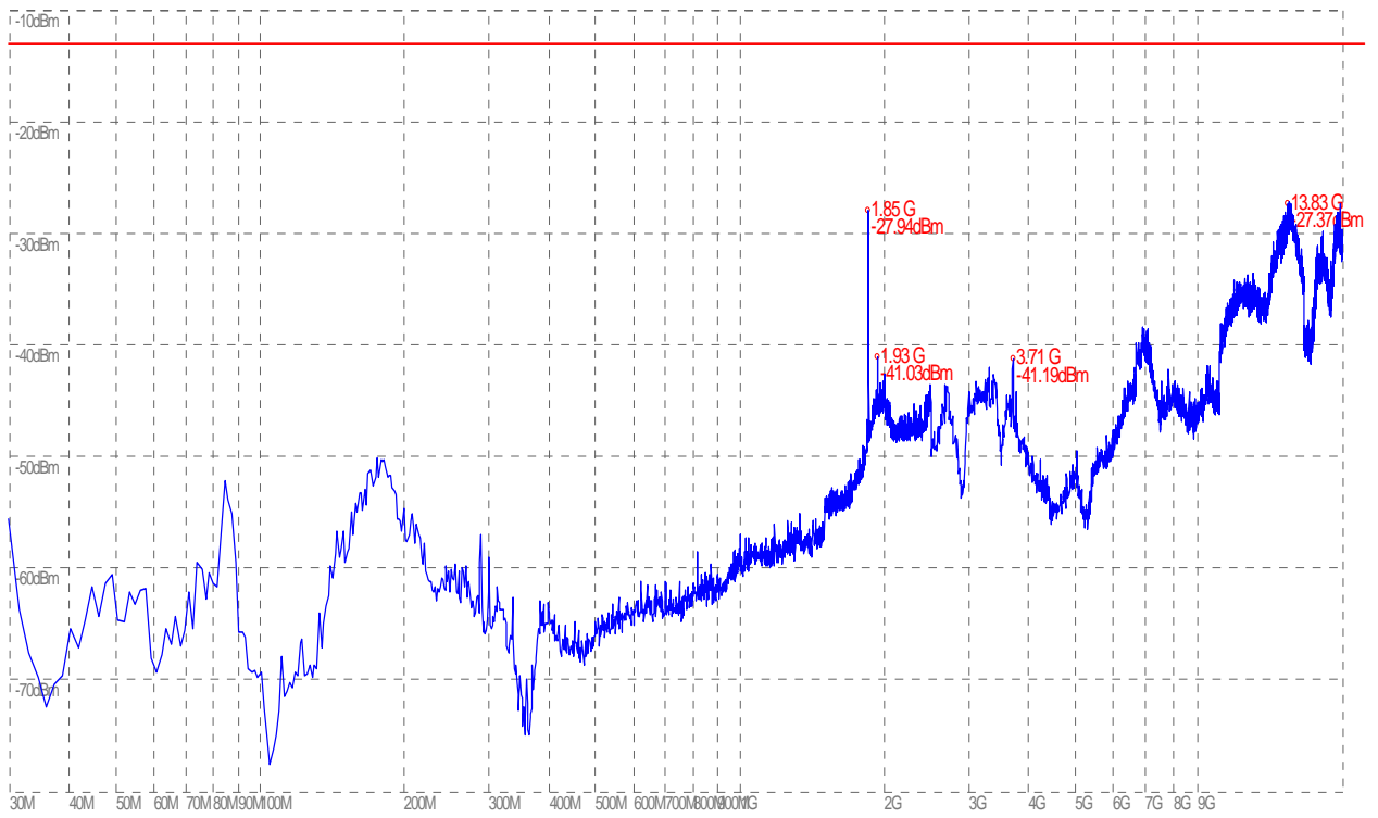
(Plot L.2: HSPA+ 1900 MHz Channel = 9662, Test Antenna Vertical)
