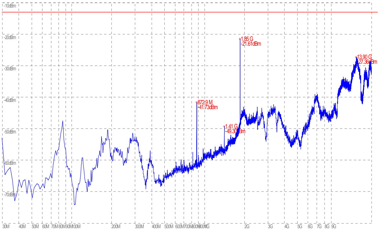
(Plot B.2: GSM 1900MHz Channel = 512, Test Antenna Vertical)
