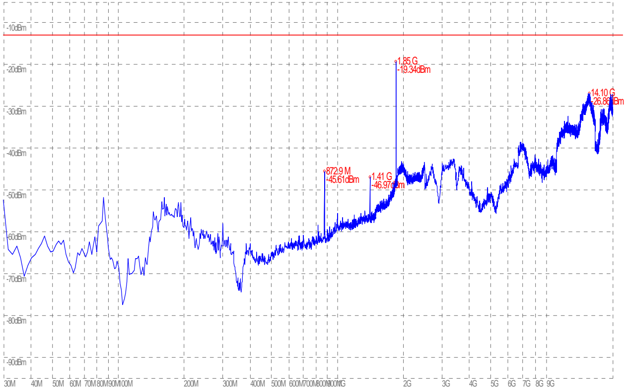
(Plot D.2: EGPRS 1900MHz Channel = 512, Test Antenna Vertical)
