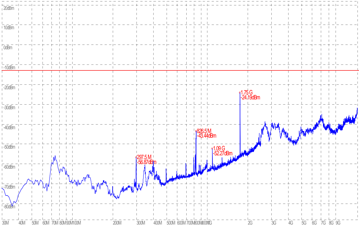
(Plot E.1: WCDMA 850MHz Channel = 4357, Test Antenna Horizontal)
