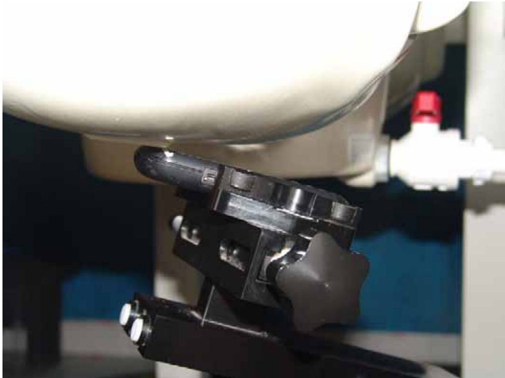
Picture B7: Right Hand Tilt 15° Position
