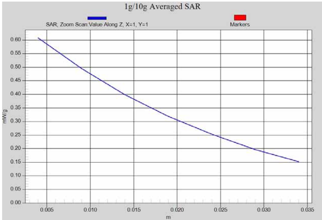
Fig. 33-1 Z-Scan at power reference point (850 MHz CH4132)
