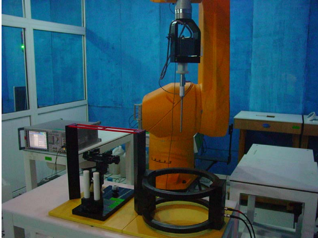
Picture A1: HAC T-Coil System Layout
