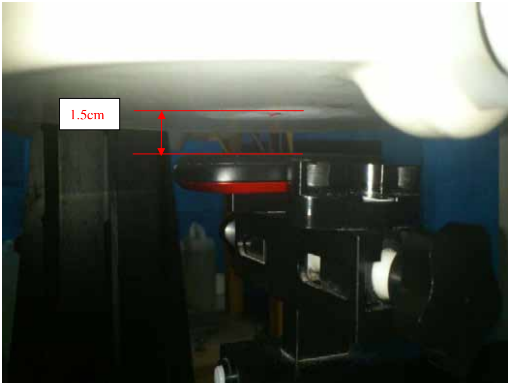
Picture B8: Body-worn Position (towards ground, the distance from handset to the bottom of the Phantom is 1.5cm)
