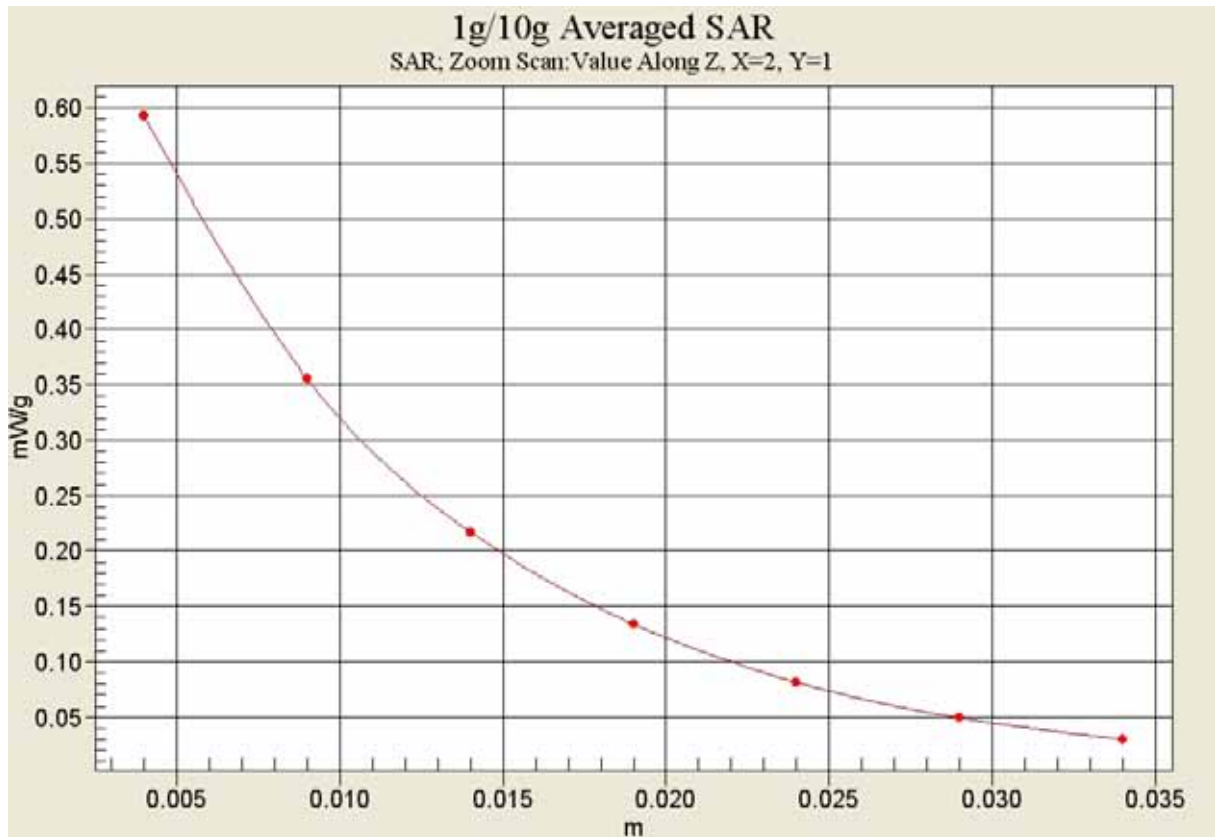
Fig. 38-1 Z-Scan at power reference point (1900 MHz CH661)
