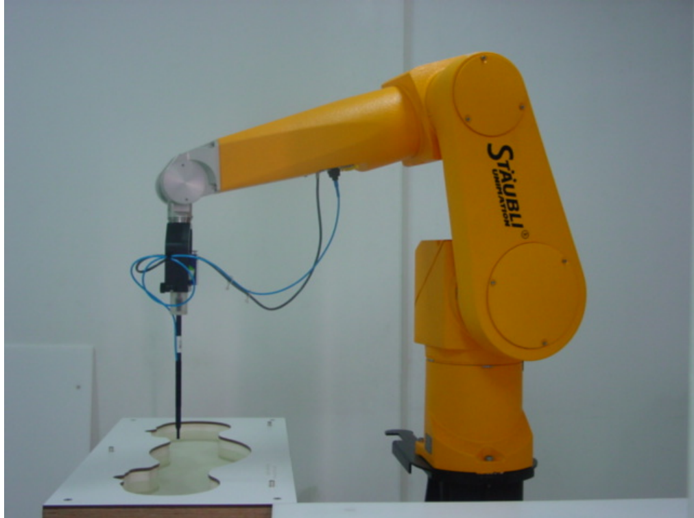
Picture B1: Specific Absorption Rate Test Layout
