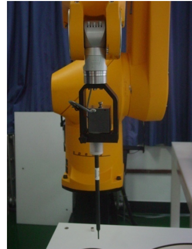
Picture4:ES3DV3 E-field probe
