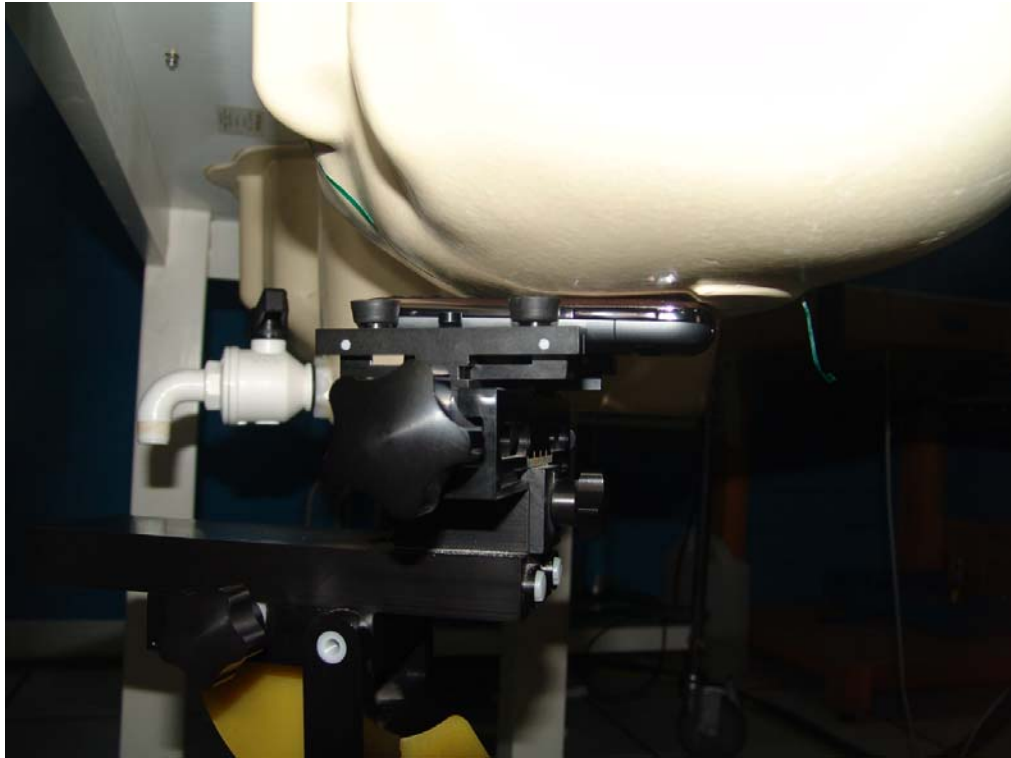
Picture B5: Left Hand Touch Cheek Position
