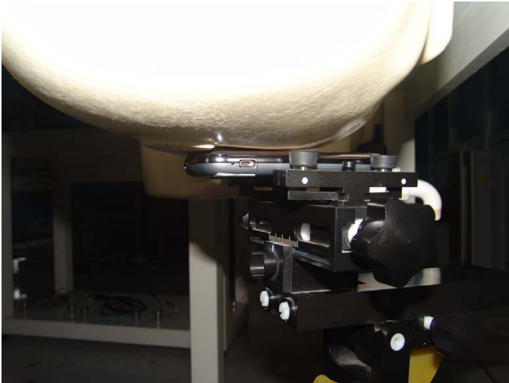
Picture B7: Right Hand Touch Cheek Position
