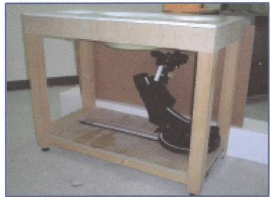
Picture 6: Generic Twin Phantom
