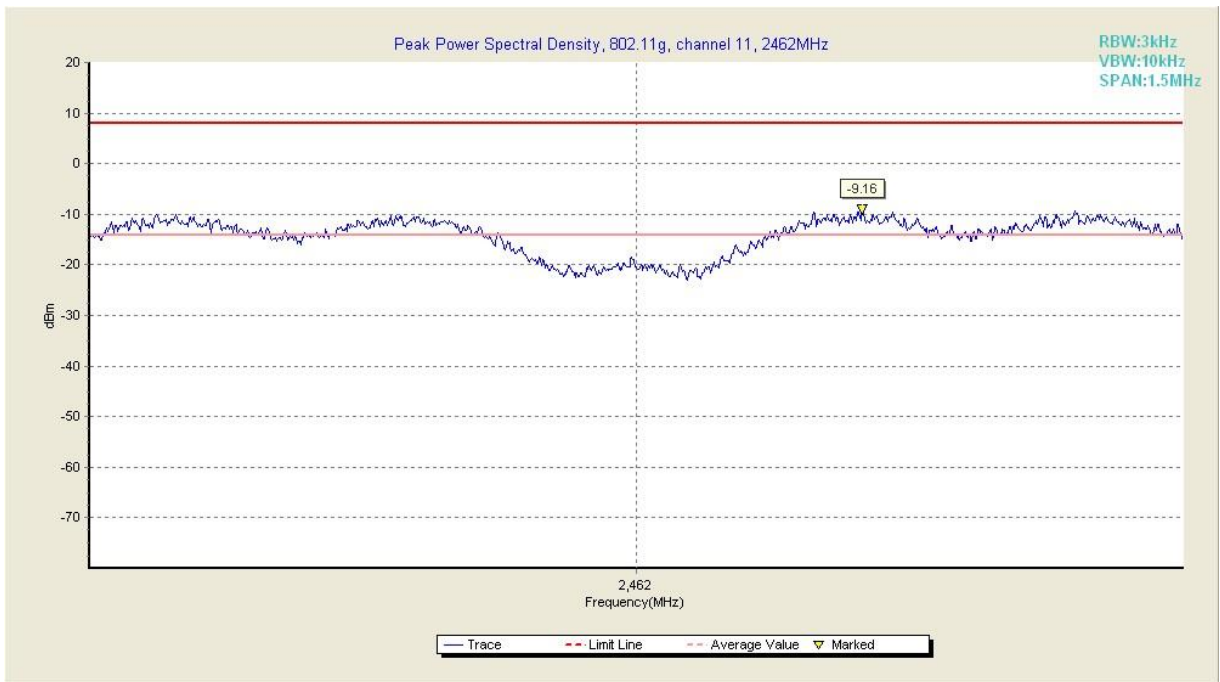
Fig. 6 Power Spectral Density (802.11g, Ch 11)
