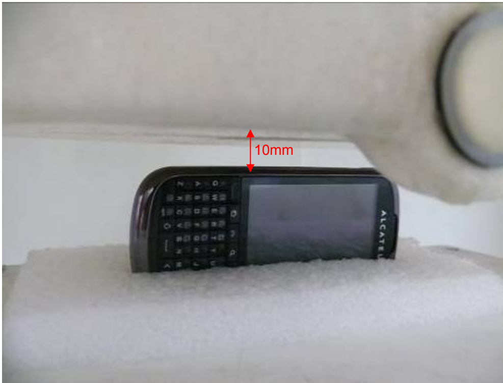
Picture 15: Left Edge, the distance from handset to the bottom of the Phantom is 10mm
