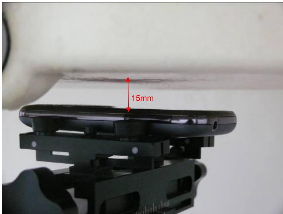
Picture 20: Front Side, the distance from handset to the bottom of the Phantom is 15mm
