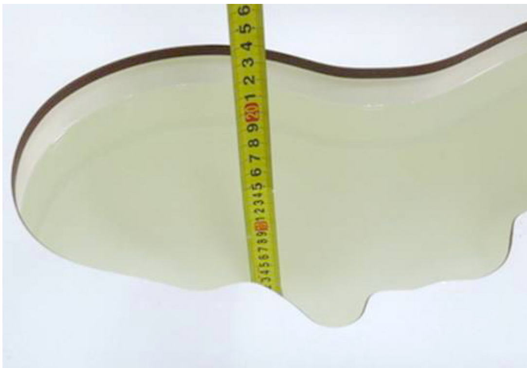
Picture 7: liquid depth in the head Phantom (2450 MHz, 15.2cm depth)
