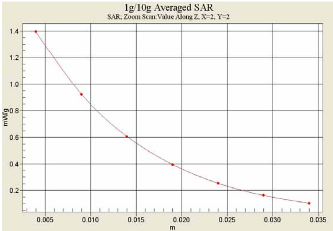
Fig. 21-1 Z-Scan at power reference point (1900 MHz CH25)
