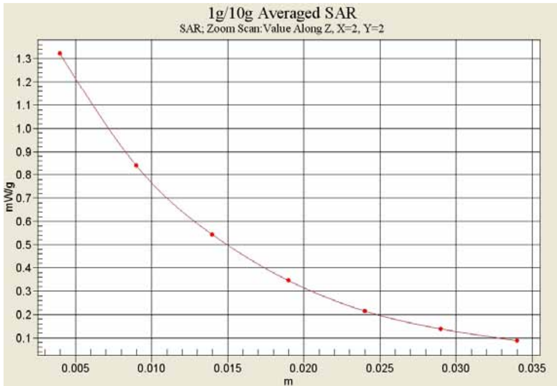
Fig. 45-1 Z-Scan at power reference point (1900 MHz CH25)
