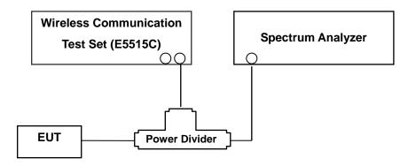
(Configuration of conducted Emission measurement)
