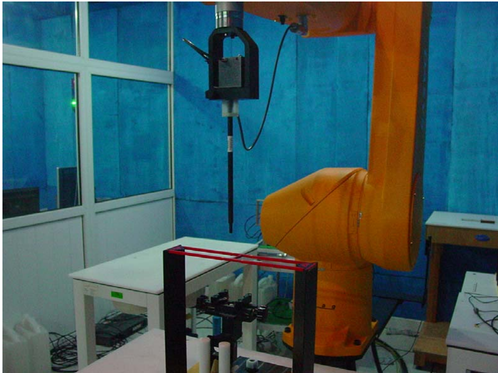
Picture A1: HAC RF System Layout
