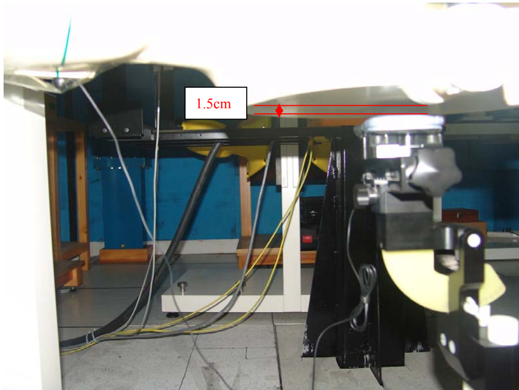
Picture B12: Body-worn Position with Headset (towards ground, the distance from handset to the bottom of the Phantom is 1.5cm) - folded
