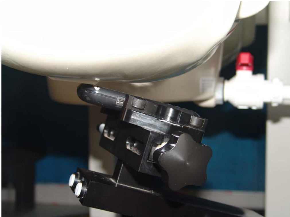
Picture B7: Right Hand Tilt 15° Position
