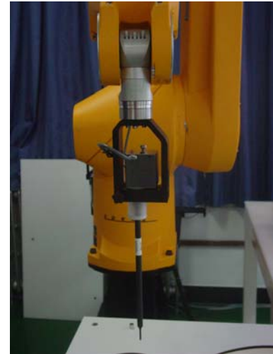
Picture4:ES3DV3 E-field probe
