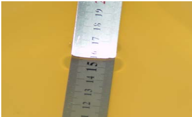
Liquid depth for SAR Measurement
