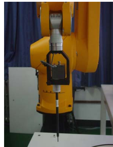
Picture4:ES3DV3 E-field probe
