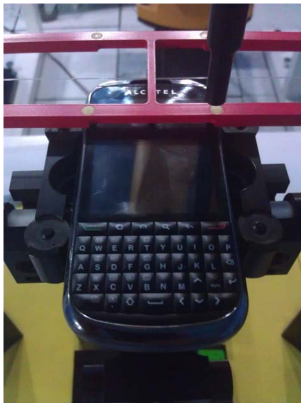
Picture 2: EUT Positioning for RF
