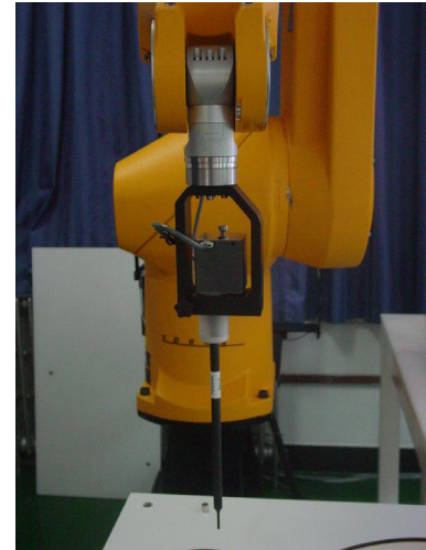
Picture4:ES3DV3 E-field probe
