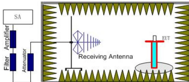
2. The EUT is then put into continuously transmitting mode at its maximum power level during the test. And the maximum value of the receiver should be recorded as (Pr).
