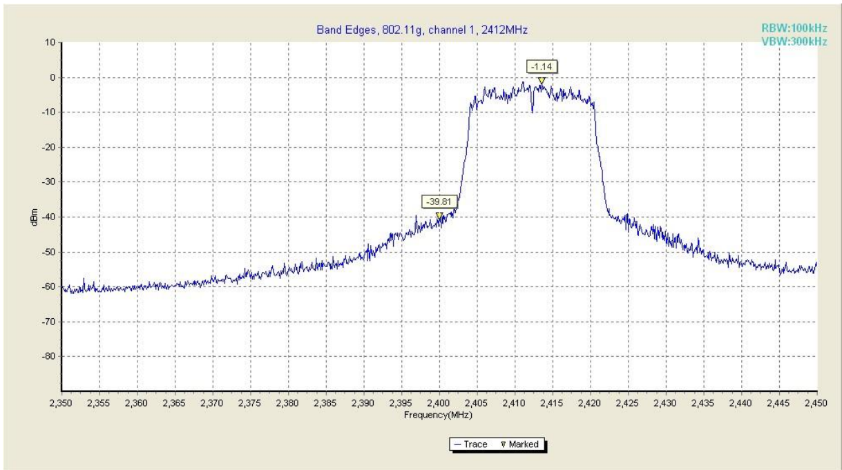
Fig. 21 Band Edges (802.11g, Ch 1)
