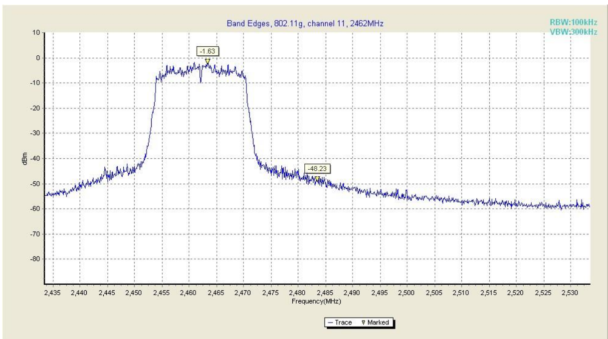
Fig. 22 Band Edges (802.11g, Ch 11)
