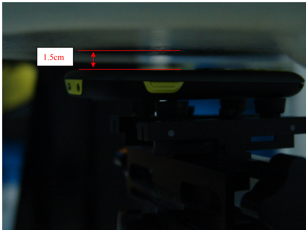
Picture B10: Body-worn Position (towards phantom, the distance from handset to the bottom of the Phantom is 1.5cm)
