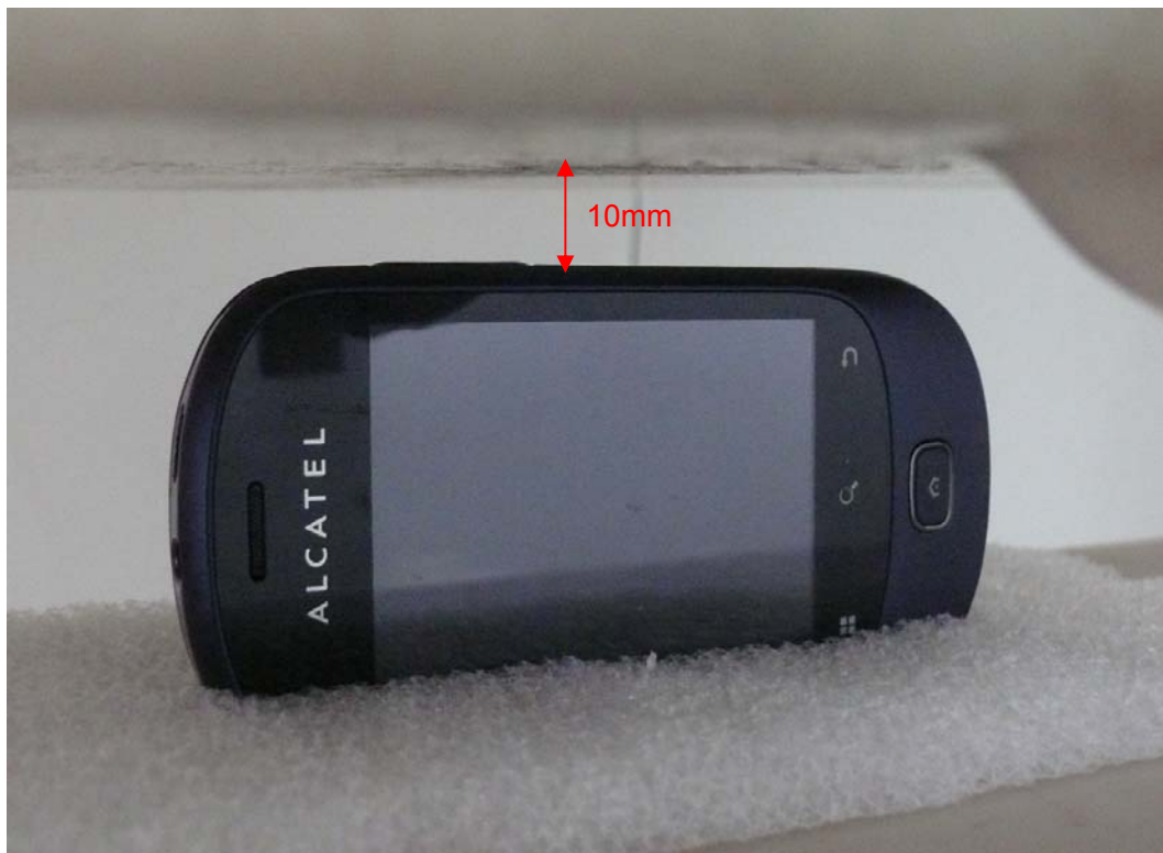
Picture 21: Right edge, the distance from handset to the bottom of the Phantom is 10mm
