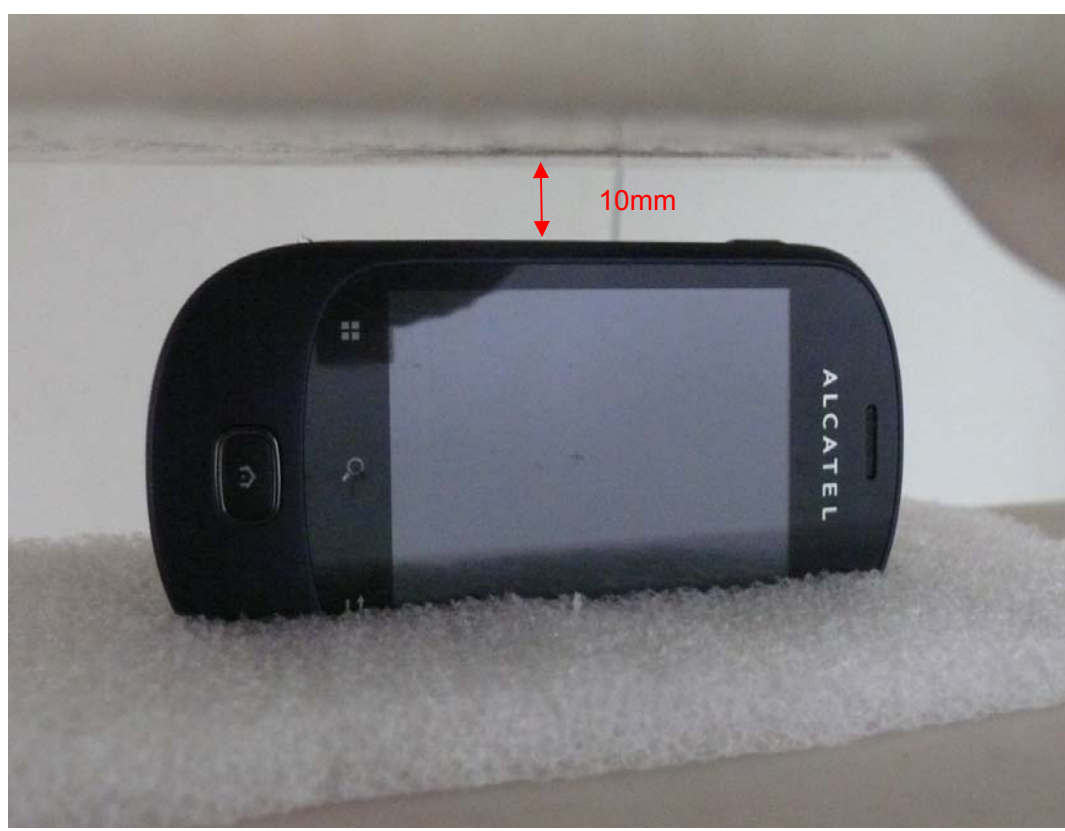
Picture 20: Left edge, the distance from handset to the bottom of the Phantom is 10mm
