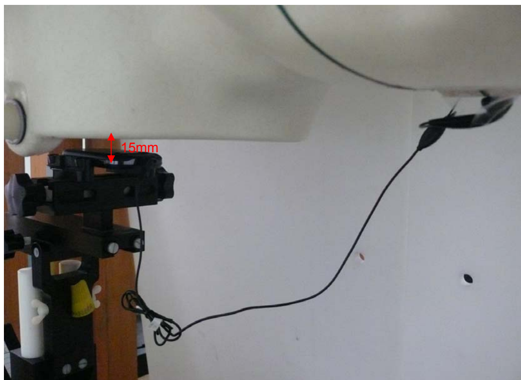
Picture 17: Body with earphone, The EUT display towards ground, the distance from handset to the bottom of the Phantom is 15mm
