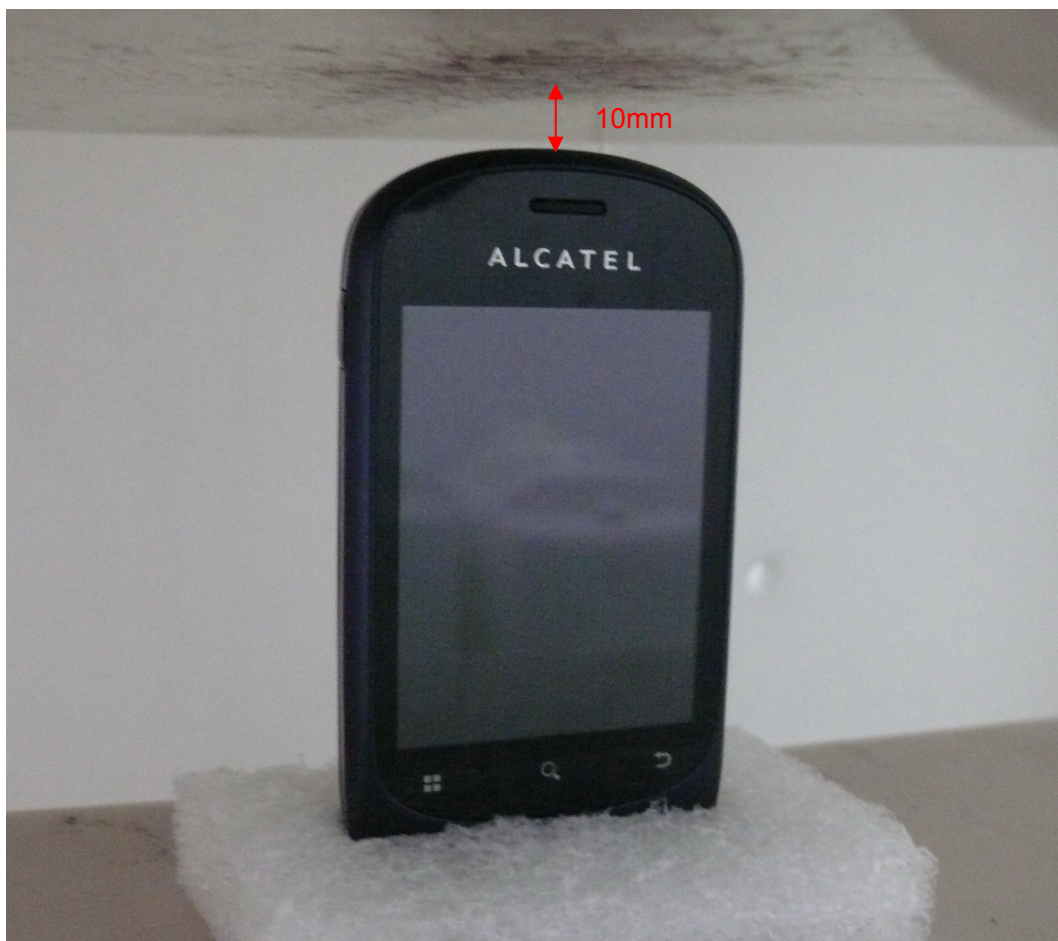
Picture 22: Top edge, the distance from handset to the bottom of the Phantom is 10mm
