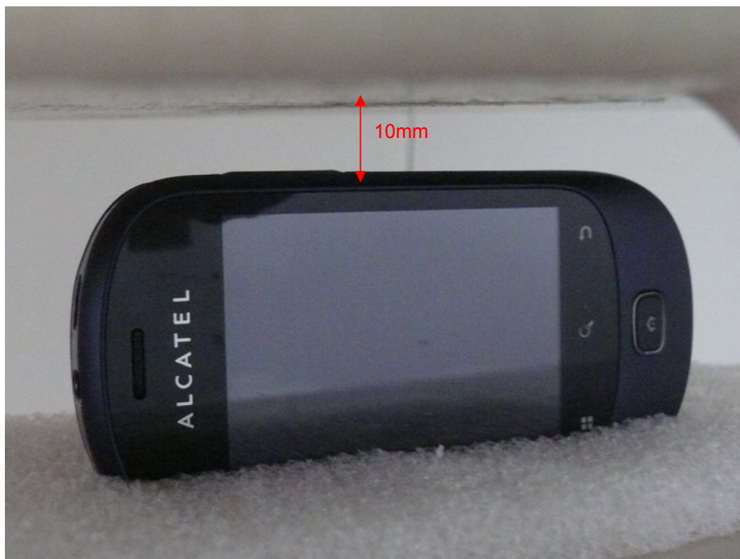
Picture 19: Right edge, the distance from handset to the bottom of the Phantom is 10mm
