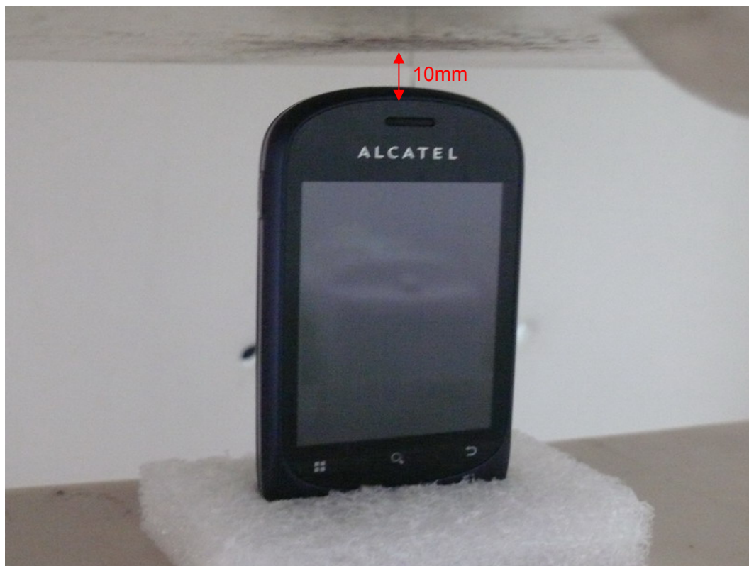
Picture 20: Top edge, the distance from handset to the bottom of the Phantom is 10mm
