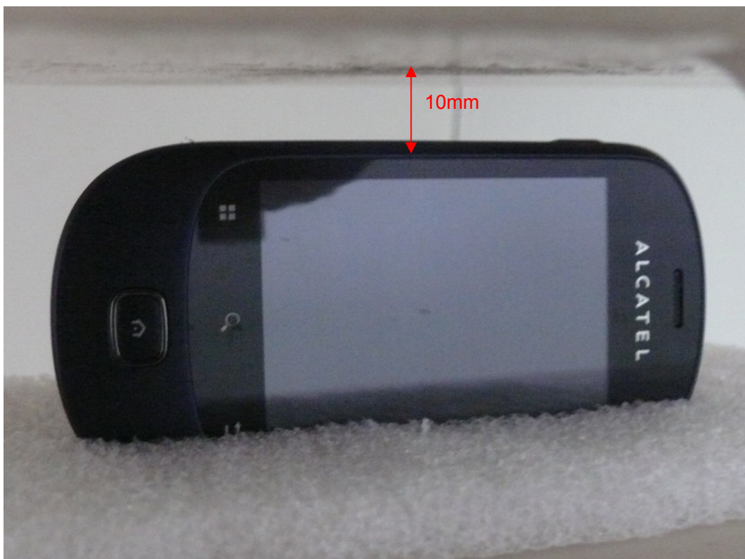
Picture 18: Left edge, the distance from handset to the bottom of the Phantom is 10mm
