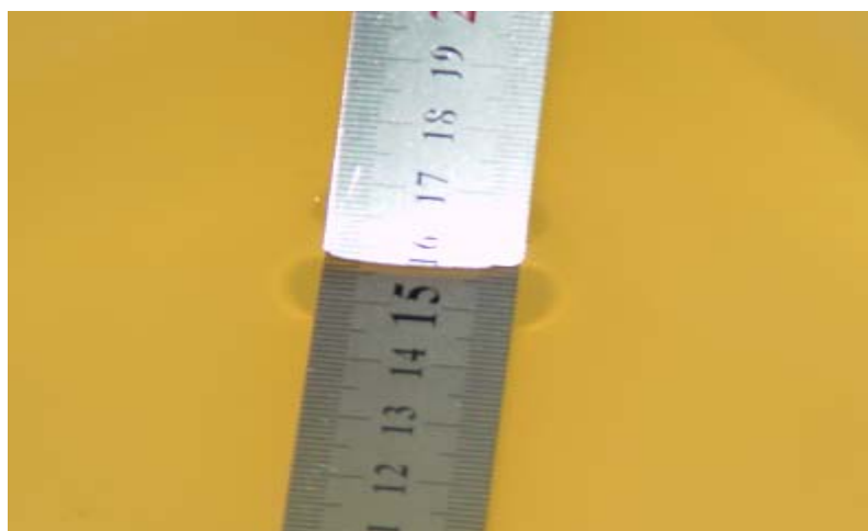
Liquid depth for SAR Measurement
