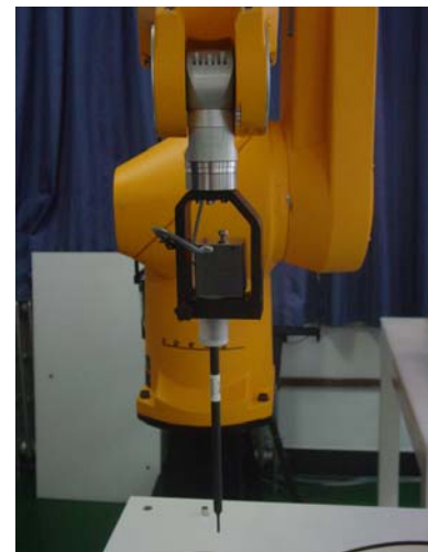
Picture4:ES3DV3 E-field probe
