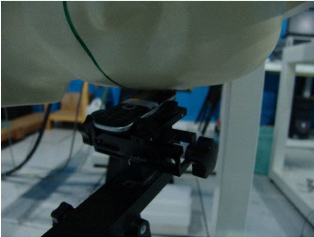
Picture B5: Left Hand Tilt 15° Position
