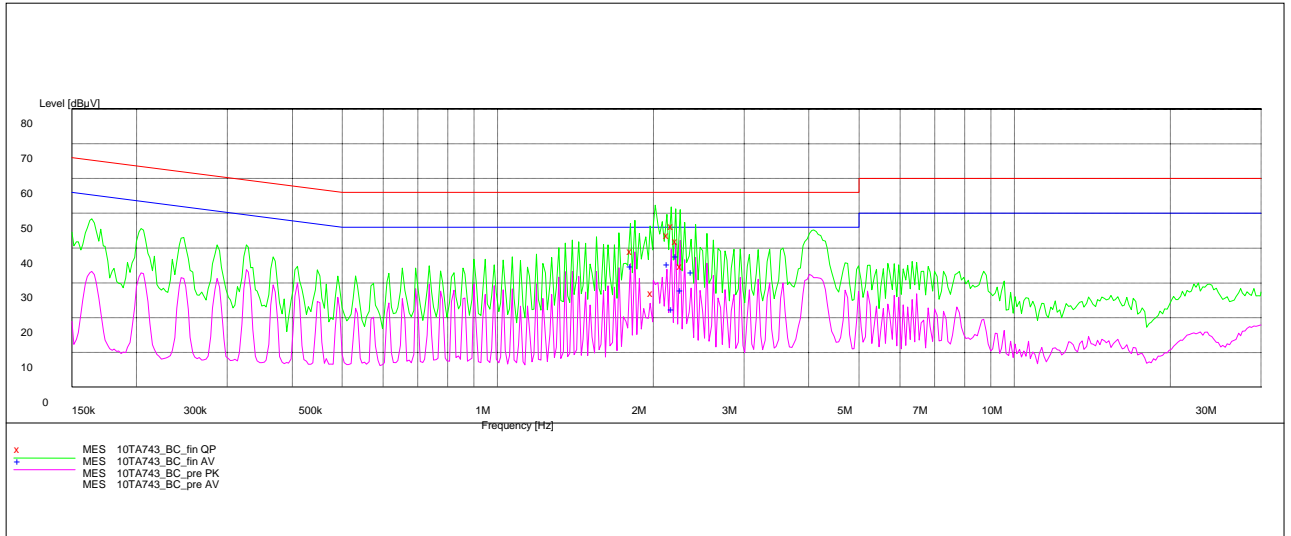
Fig.37 AC Powerline Conducted Emission with charger
