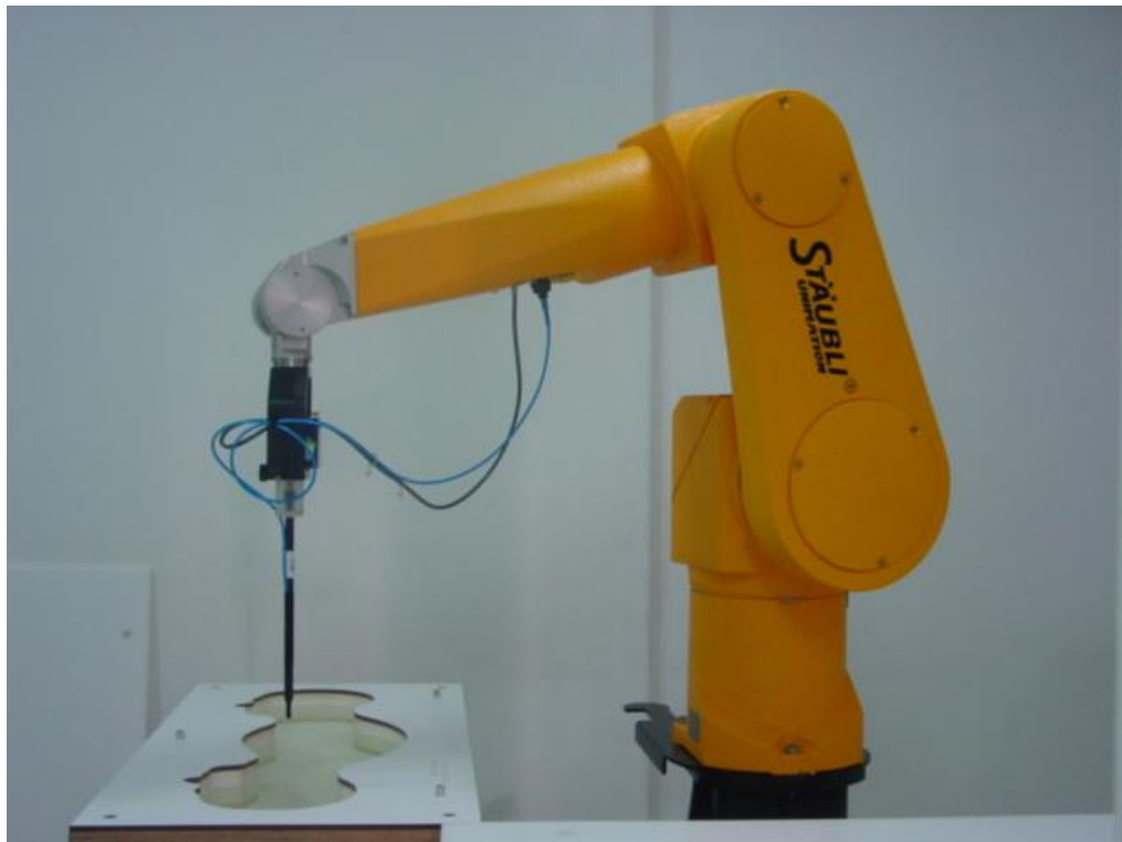
Picture B1: Specific Absorption Rate Test Layout
