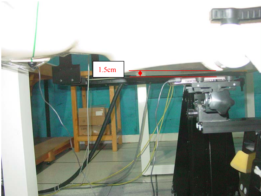
Picture B11: Body-worn Position with Headset (towards ground, the distance from handset to the bottom of the Phantom is 1.5cm)
