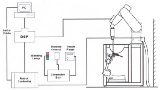
Picture 2: SAR Lab Test Measurement Set-up
