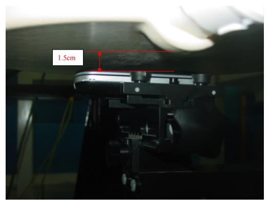
Picture B9: Body-worn Position (towards phantom, the distance from handset to the bottom of the Phantom is 1.5cm)
