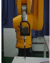
Picture4:ES3DV3 E-field probe
