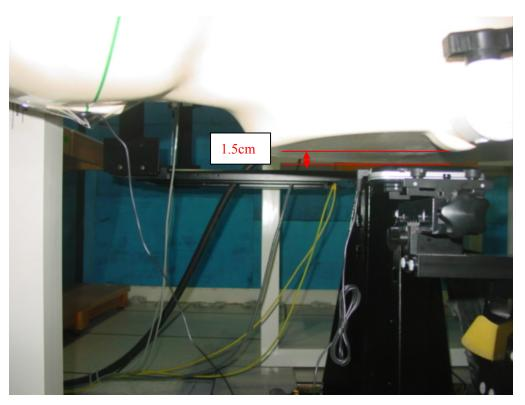
Picture B10: Body-worn Position with Headset (towards ground, the distance from handset to the bottom of the Phantom is 1.5cm)
