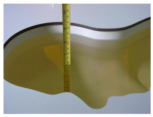
Picture B2: Liquid depth in the Flat Phantom (850 MHz)
