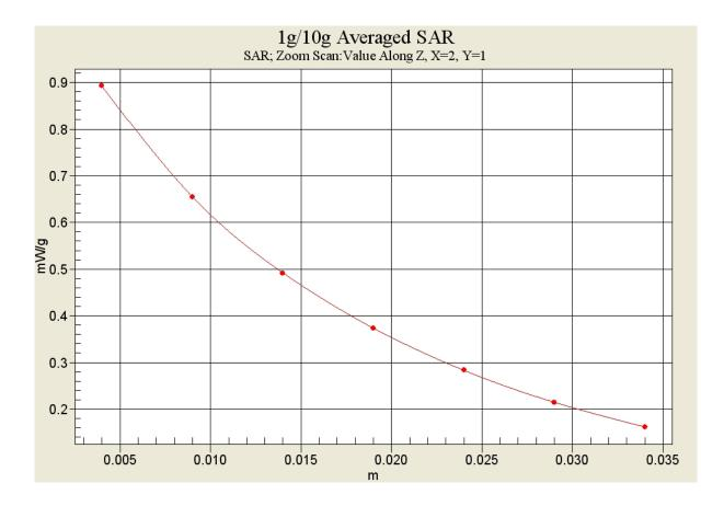
Fig. 7-1 Z-Scan at power reference point (850 MHz CH251)
