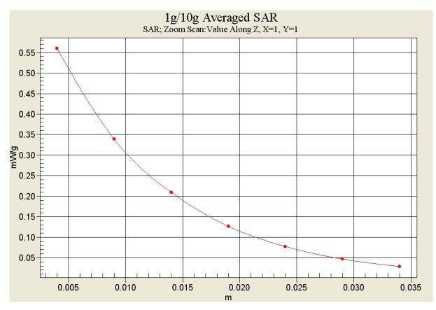
Fig. 34-1 Z-Scan at power reference point (1900 MHz CH661)
