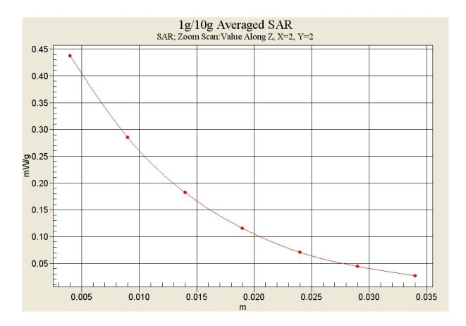
Fig. 20-1 Z-Scan at power reference point (1900 MHz CH661)
