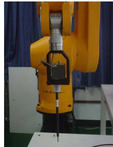
Picture4:ES3DV3 E-field probe
