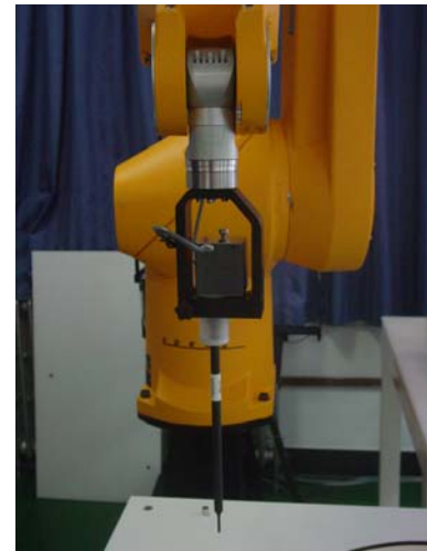
Picture4:ES3DV3 E-field probe
