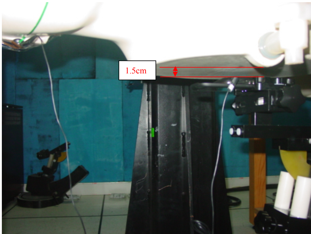
Picture B19: Body-worn Position with Headset (towards ground, the distance from handset to the bottom of the Phantom is 1.5cm) – Slide up
