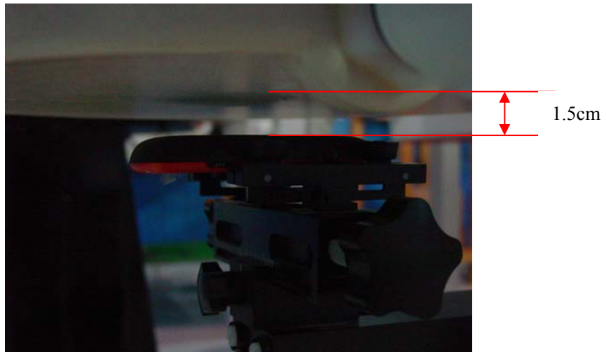
Picture B11: Body-worn Position (towards ground, the distance from handset to the bottom of the Phantom is 1.5cm)
