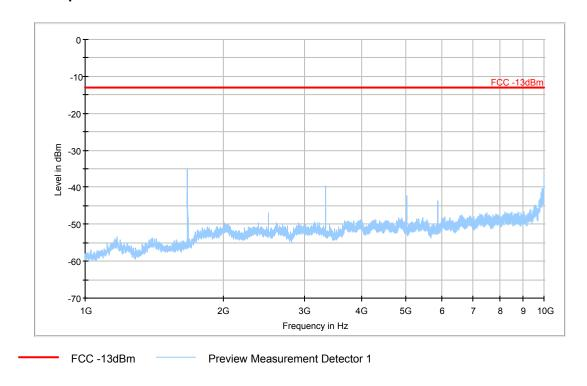
A.2.3.6 RADIATED SPURIOUS EMISSIONS-Channel 251: 1GHz – 10GHz Radiated spurious emission limit :-13dBm.
