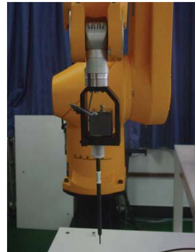
Picture4:ES3DV3 E-field probe
