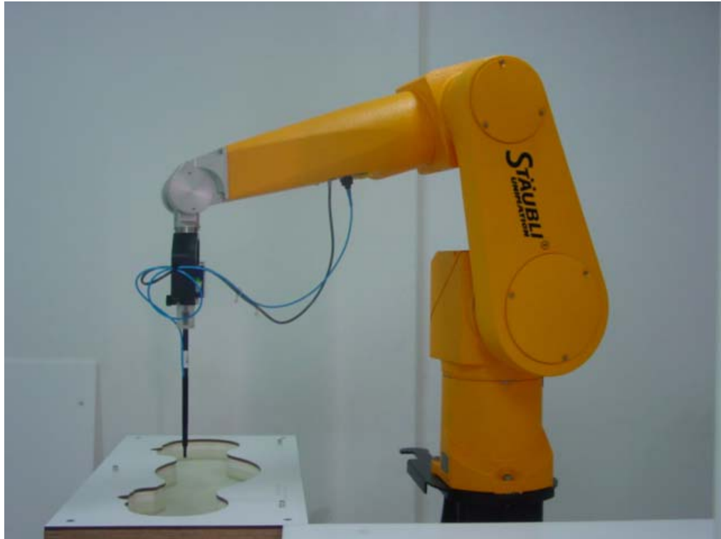
Picture B1: Specific Absorption Rate Test Layout
